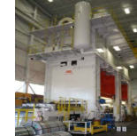
Clearing Transfer Press - Provides ability to layout complete sets of the transfer dies under one ram for production emulation
